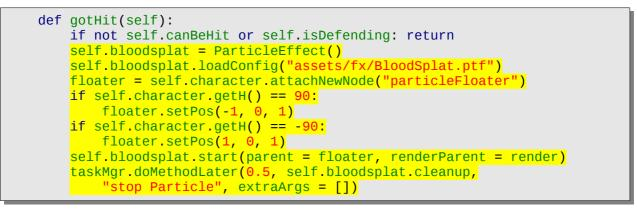
The first lines are there for instantiating and loading the particle effect. The floater will be used to place the effect respective to the character so it will be visible in front of it. After that we start the particle effect and start a task so the effect get stopped and removed half a second later.
