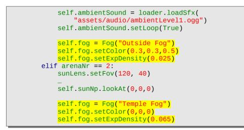
This will add a simple exponential fog that will move with the camera and have its density raised from the camera into infinity by the given setExpDensity value.
